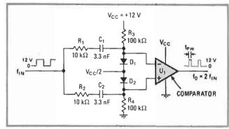
**Doubler.** Single comparator  $U_1$  and a few discrete components yield a frequency doubler that generates a positive pulse of duration  $t_{pw}$  on both the rising and falling edges of the input signal. The duration of the pulse  $(t_{pw})$  is adjustable and is given by  $K(R_1+R_3)C_1$  for the falling edge and  $K(R_3+R_4)C_2$  for the rising edge. For the components shown,  $t_{pw}$  measures about 0.31 ms.
