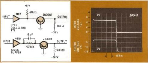
1. Level translator. A field-effect transistor in the commongate configuration can provide output voltages that are higher than the supply voltage of the driving logic. Here the FET voltage-shifter accepts input levels of 0 or 3 V and delivers outputs of 0 or 10 V. The fast transitions and short delays that are demonstrated in the oscilloscope photo are achieved by minimizing the load capacitance.
