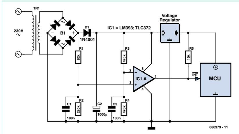
have only added an extra diode (D1) in the main supply path. In normal operation smoothed DC levels appear at the output of the voltage dividers, and hence at the inputs to comparator IC1. The component values in the first voltage divider (R1, R2 and C1) must be selected so that its output voltage, in the range 0.5 V to 1 V, is a little higher than that of the second
