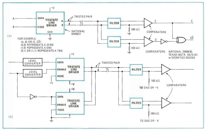
**Getting more out of a twisted pair.** Ternary-coded data can be transmitted at megabit rates through ordinary twisted pairs over long distances. A single integrated tristate line driver can be used to send the data at low bit rates, as in (a); or two drivers can be employed, as in (b), for higher bit rates. If desired, the third state can be used for synchronization purposes or to transmit status or control information.
