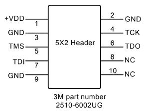
Figure 11. Header Connection Example
