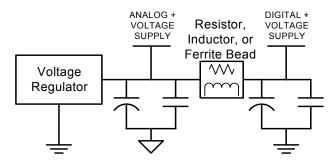
Figure 5. Filtering Analog Power Supply
