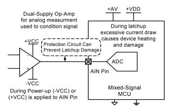
Figure 19. Example Latchup Potential
