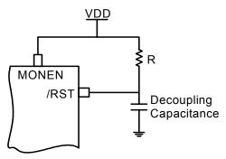
Figure 10. Decouple and Pull-Ups on the RST and MONEN Lines
