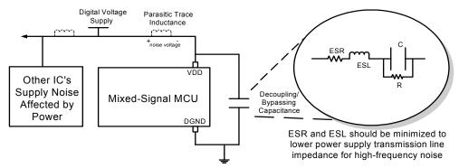
Figure 17. Local Decoupling and Bypassing Circuit
