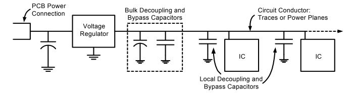
Figure 1. Typical Components of a PCB Power Supply
