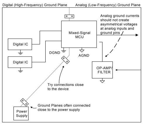
Figure 7. Placing Microcontroller on both Analog and Digital Ground Planes
