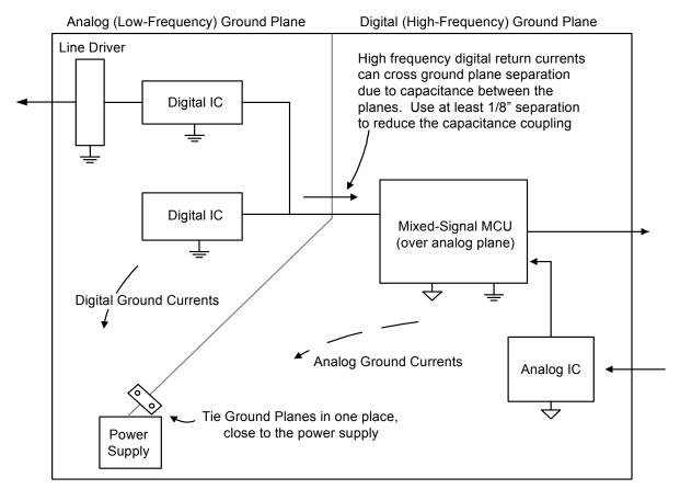
Figure 6. Using Split Analog and Digital Ground Planes
