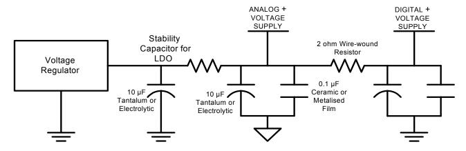
Figure 2. PCB Power Supply Circuit with Decoupling, Bypassing, and Isolation
