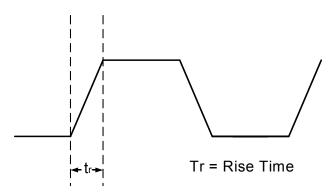
Figure 16. Digital Waveform Rise Time
