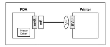
Figure 3. OTG cable is inserted "backwards".
