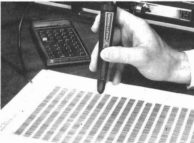
Fig. 1. Hewlett-Packard's bar code-reading Optical Wand plug into an HP-41C calculator.
