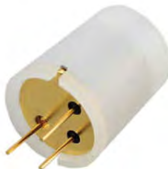
Fig.4. The EKMC1601113 digital output PIR sensor from Panasonic Electric Works
