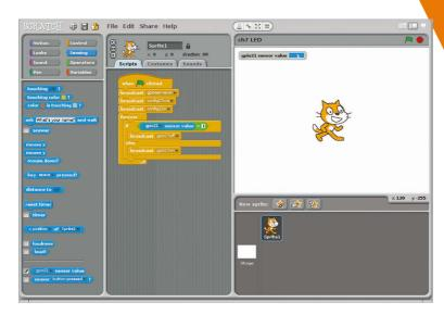
Left: Ticking the button's gpio21 sensor value will show it on the stage, which is handy for testing
