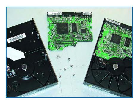
ing ahead), we tried it with the new type, but the old drive protested loudly, with the heads apparently moving all over the place. The only positive aspect of our first attempt was that it established that the internal discs could still rotate. The motor itself was therefore not broken.
