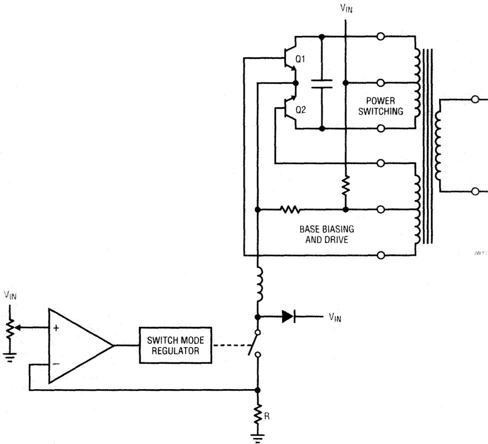
**Figure 11-12.** Switched mode current sink restores efficiency.
