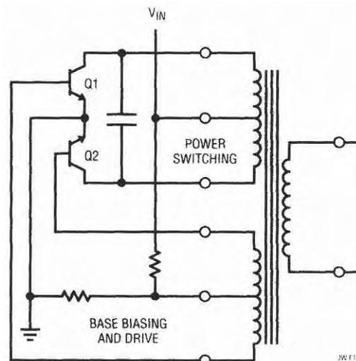
**Figure 11-10.** Adding the resonating capacitor to the Royer.
