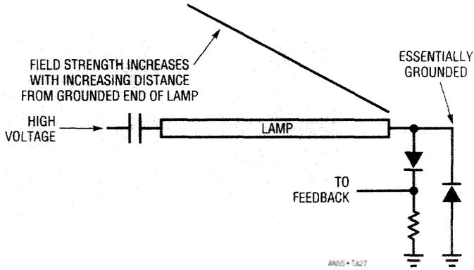
**Figure 11-34.** The "low thermometer" configuration. "Topside sensed" primary derived feedback balances lamp drive, extending dimming range.
