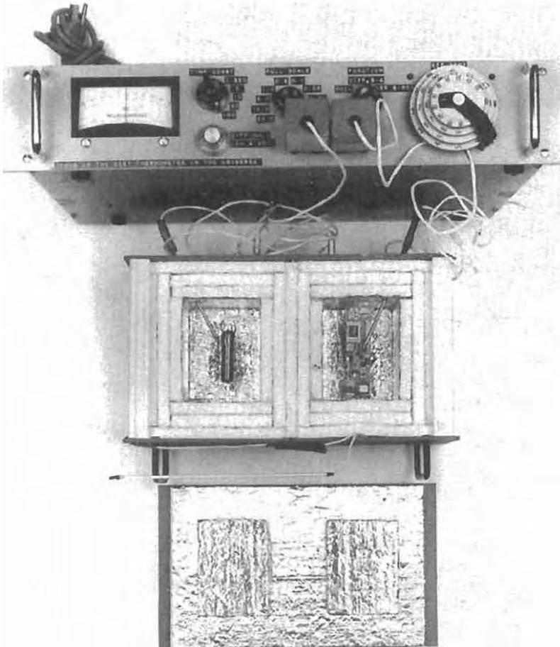
**Figure 11-A9.** The calorimeter (center) and its instrumentation (top). Calorimeter's high degree of thermal symmetry combined with sensitive servo instrumentation produces accurate efficiency measurements. Lower portion of photo is calorimeter's top cover.
