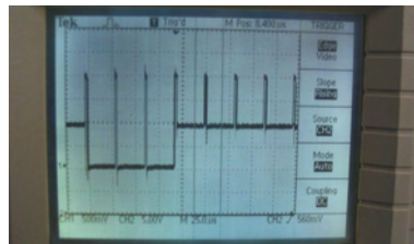
Figure 2 Applying the diode-gated composite-synchronization waveform to a 75Ω load results in clean synchronization pulses.
