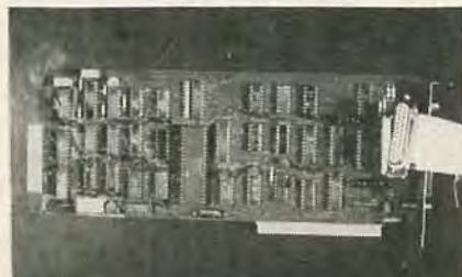
FIG. 12—THE FLOPPY-DISK CONTROLLER adapter shown here also comes equipped with a parallel printer port.
