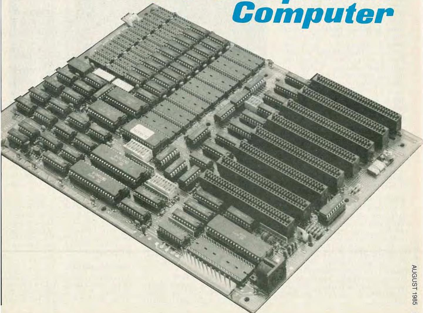
pending on how many floppy-disk drives are installed. For 1 drive, both should be on. For 2 drives, SW1-7 should be off, but SW1-8 should be on. For 3 drives, SW1-7 should be on, but SW1-8 should be off. For 4 drives, both should be off.
