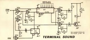
NTENDED as an addition to microprocessor or VDU keyboards, this produces a different pattern of high and low tones for each key on the keyboard. Although it is not necessary to learn these different patterns, after some use the tone generator becomes a real aid to accurate
