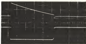
Fig. 19. Gate waveform (top) 5V/cm. TR2 collector (bottom) 5V/cm. Time 0.5 second per centimetre. (Refer to Fig. 18)
