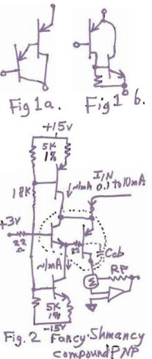
It turns out that this trick circuit has some advantages (Fig. 2). It not only has better alpha than the best single PNP, it also has lower output capacitance and faster F-alpha. These days, PNPs are often good enough so you don't always get in trouble with them. But sometimes, this circuit's advantages are still useful.
