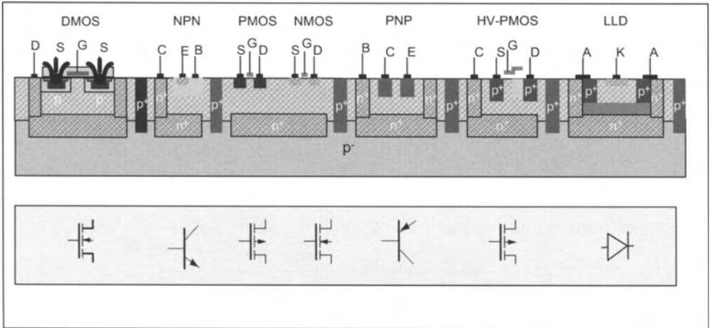
*Fig. 2.2: Cross section of some devices of an SPT technology*
