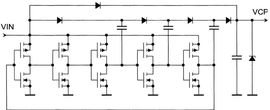
Fig. 4.4: Charge pump circuit
