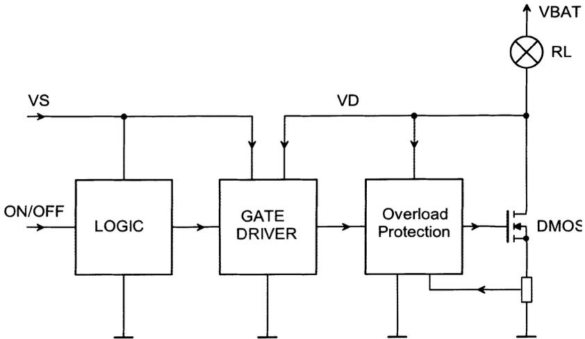
*Fig. 4.2: Block diagram of the lamp driver circuit*
