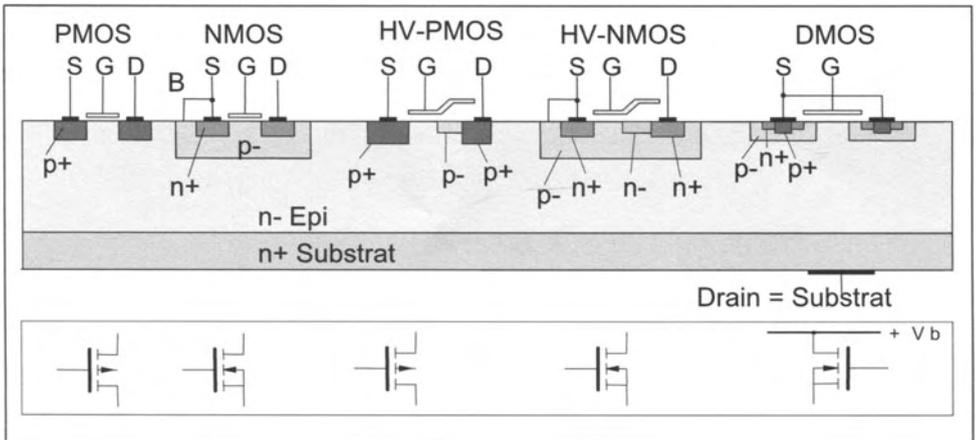
Fig. 2.1: Cross section of vertical Smart Technology
