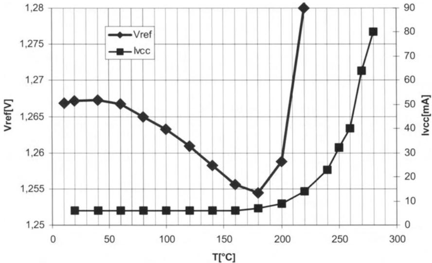
Fig. 3.2: Standard bandgap reference circuit performance and total current consumption
