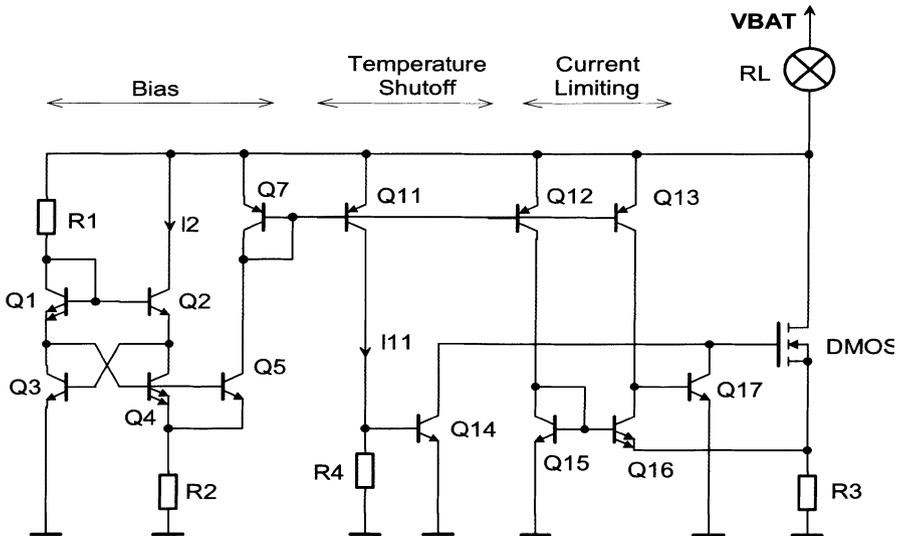
Fig. 4.5: Overload protection circuit
