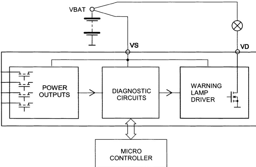
*Fig. 4.1: Block diagram of a smart-power system chip*
