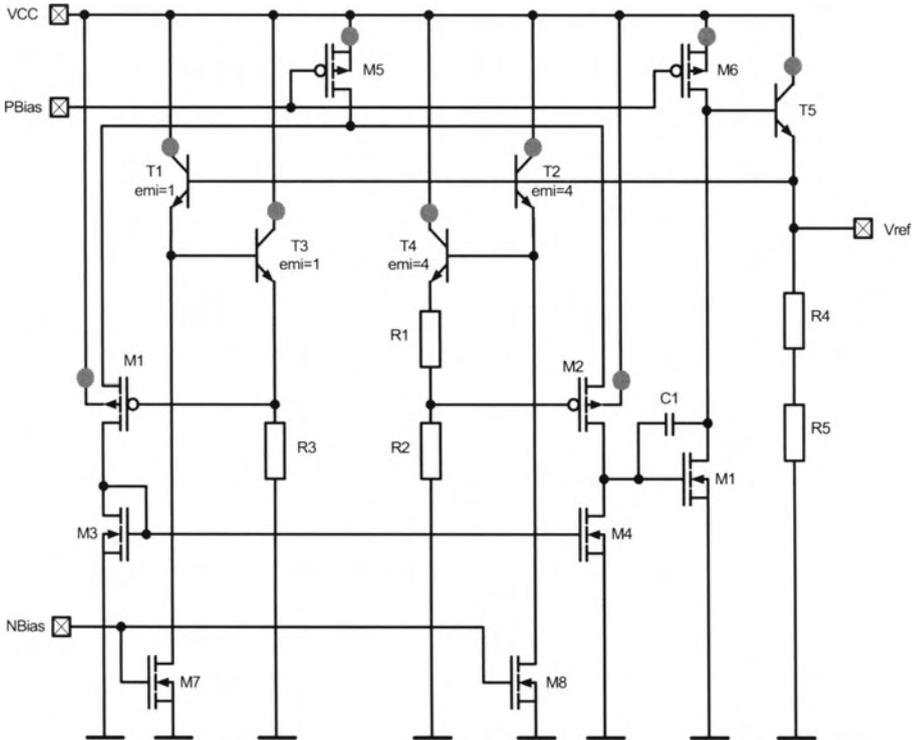
*Fig. 3.3: Robust bandgap reference – simplified schematic*
