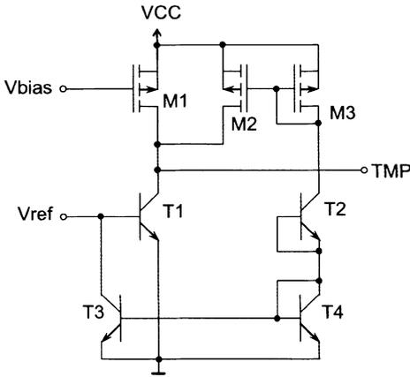
Fig. 5.3: Temperature sensor with full leakage current compensation
