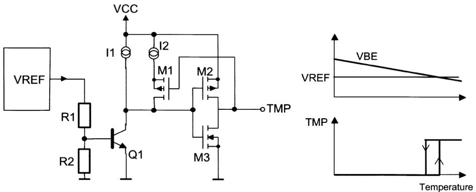
Fig. 5.1: Temperature sensor with hysteresis
