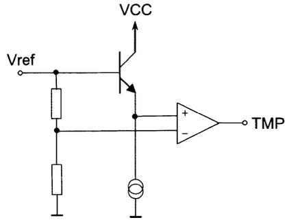
Fig. 5.4: Temperature sensor with collector at supply line t
