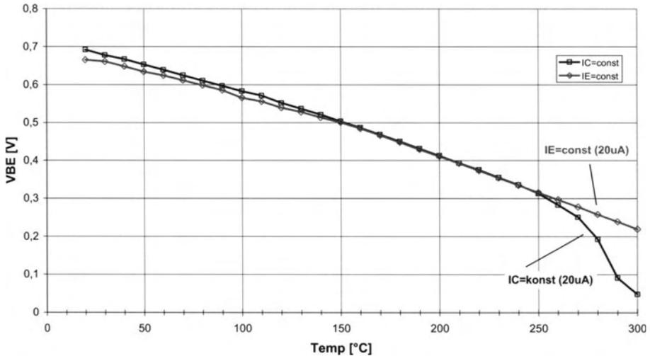
*Fig. 5.2: Measured data of base-emitter voltage vs. temperature*
