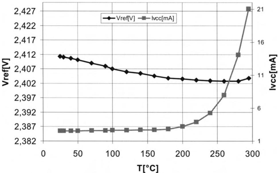
Fig. 3.4: Robust bandgap reference – measurement result
