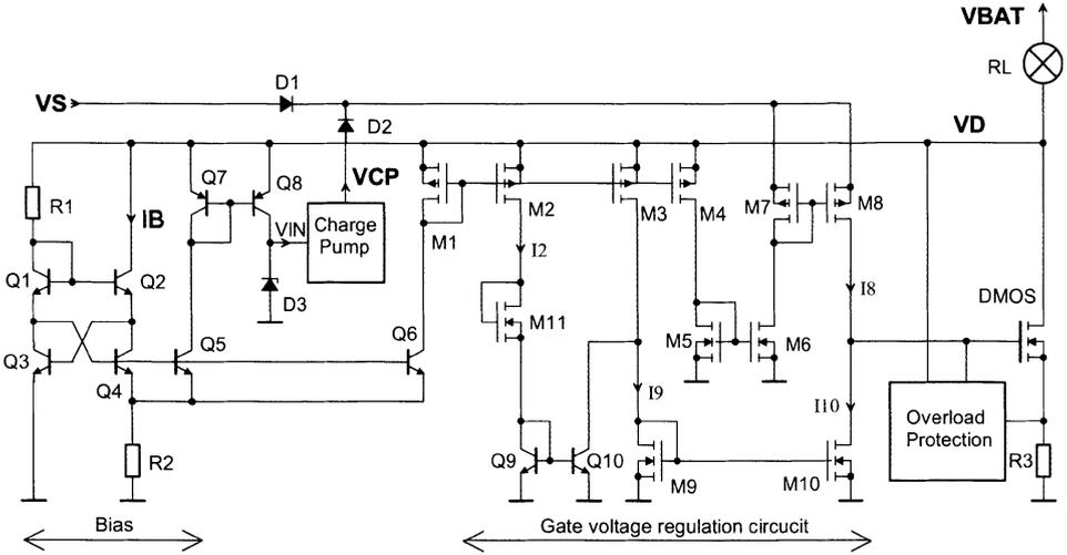
Fig. 4.3: Circuit diagram of the lamp driver circuit
