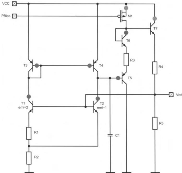
Fig. 3.1: Brokaw cell with substrate junctions (red circles)
