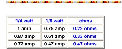
Example if you need a 3/4 amp fuse use a 0.47 ohm 1/4 watt resistor.
