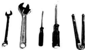
TYPICAL TOOLS REQUIRED FOR SYTEN & SEASTAR CYLINDER SEAL OVERHAUL.
