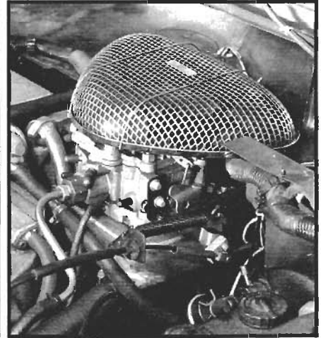
A Rochester two-barrel carburetor meters fuel to the hot-vapor engine in the test Horizon.
