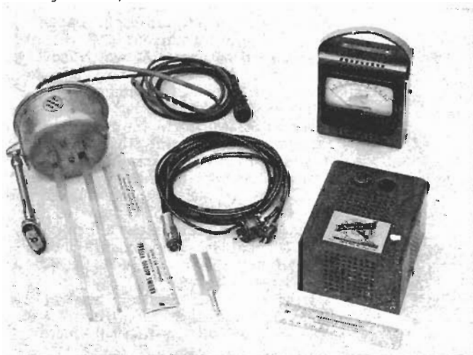
Fig. 9. Complete X-band radar. Note dielectric antenna rods.
