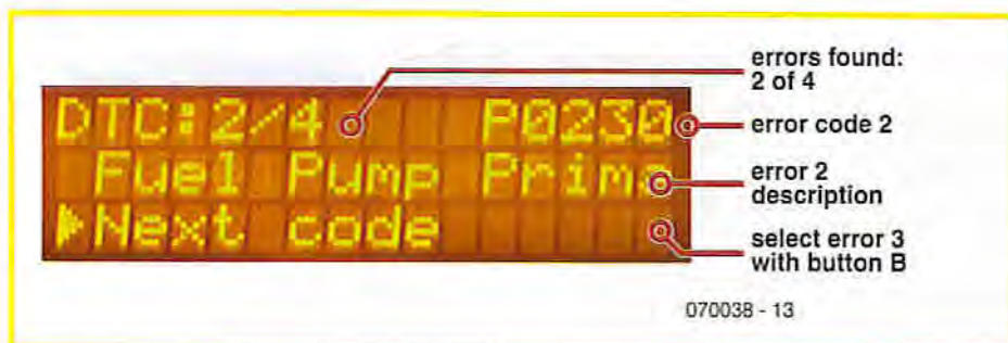
Figure 10. Trouble code menu showing a description of the trouble in running text.
