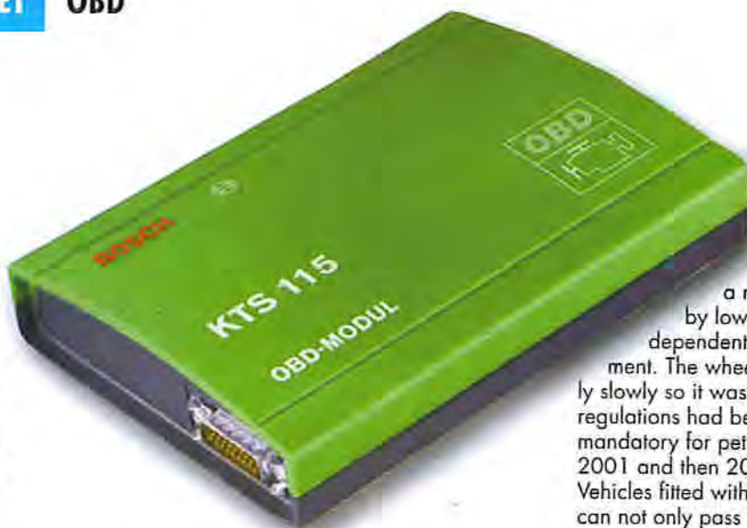
Figure 2. An OBD-Analyser. The Bosch KTS 115 is a handheld device similar to the stand-alone OBD analyser feature in this magazine.
