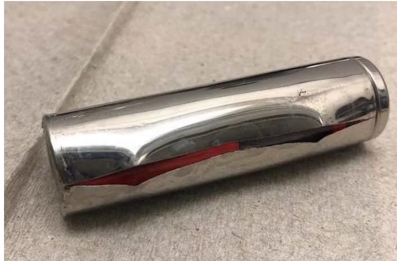
A lithium-ion EV battery that cracked after fast charging. Image used courtesy of Ozkan Lab/University of California, Riverside .
