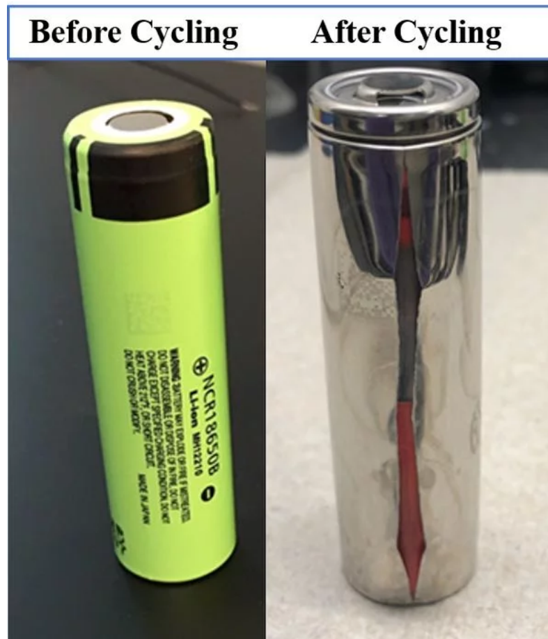
An EV battery before and after undergoing fast charging. Image used courtesy of O:kan Lab/University of California, Riverside .
