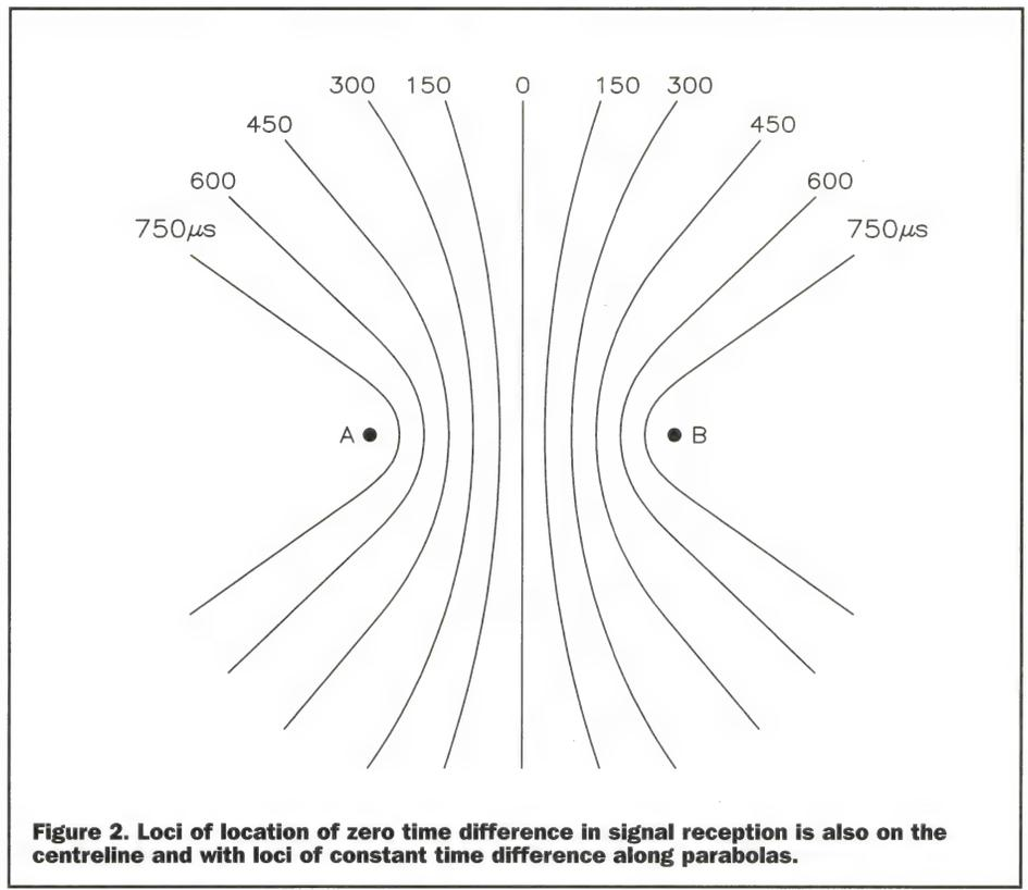
Figure 2. Loci of location of zero time difference in signal reception is also on the centreline and with loci of constant time difference along parabolas.
