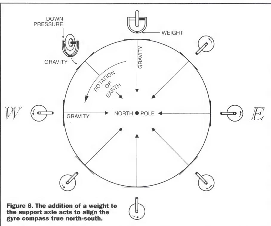
**Figure 8. The addition of a weight to the support axle acts to align the gyro compass true north-south.**
