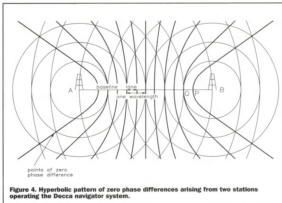
Figure 4. Hyperbolic pattern of zero phase differences arising from two stations operating the Decca navigator system.
