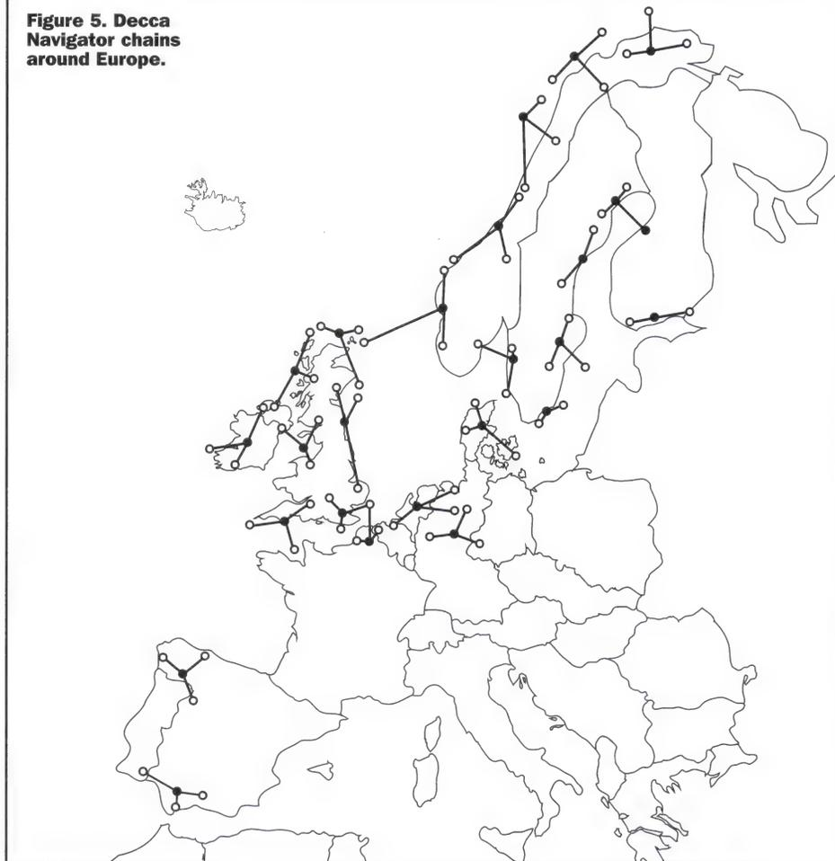
however, allows each transmitter in turn to broadcast all the frequencies of the chain at the same time. This allows the relative phase of a signal at fundamental frequency  $f$  to be derived – in the case of the red chain, identifying lanes of width 10.5km wide. This in turn allows lane count to be re-established if lost. Figure 5 indicates the Decca Navigator chains around Europe.
