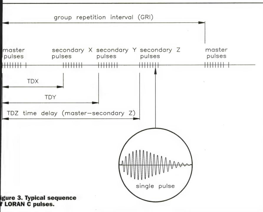
Figure 3. Typical sequence of LORAN C pulses.
