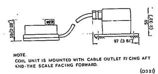
Supply Voltage: 10.5v stabilised; Weight: 1.0Kg; Cable Supplied: 1m to connector box, 4 way x 7/0.1mm; 2m main cable, 3 way x 16/0.2mm; Environmental Classification: Not splashproof, and should be mounted under cover from direct spray. Compass Safe Distance: Coil Unit - Not applicable; Box: Grade 1, 300mm (12 ins); Grade 2, 300mm (12 ins).
