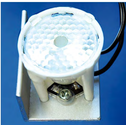
Figure 7. The LED (mounted on its carrier board) and lens are bolted to a piece of aluminium angle to make the lighting module.
