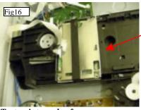
If the shorting PCB seen in Fig 3 is not in place, you will need to keep the DSP still connected to CN501 connector until pick-up shorting is done as seen on figure 10. Keep DSP attached to the frame with an electrical tape.
