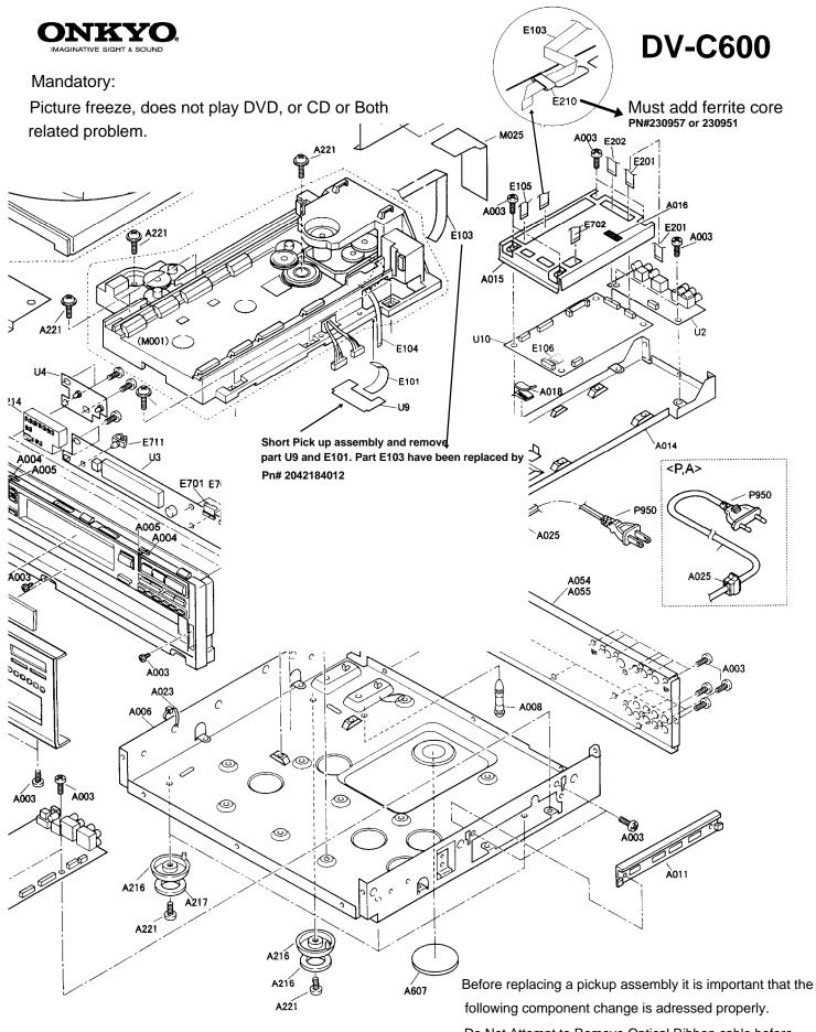
Do Not Attempt to Remove Optical Ribbon cable before shorting the landing found on the pick-up Assembly.
