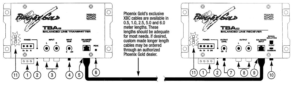
Quick Disconnect Power Plug: This connector is easily unplugged for servicing wiring connections and contains the following terminals: B+ Terminal (Battery Positive): Connect to the stereo's power distribution system that is connected directly to the positive battery terminal.
