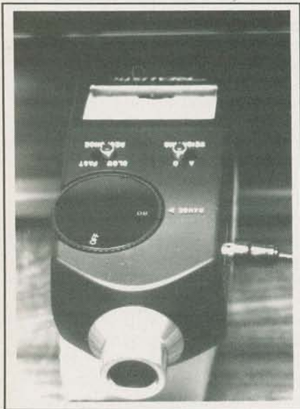
The output of the meter is fed into a scope; at the moment it's reading the whirring of the camera shutter.
