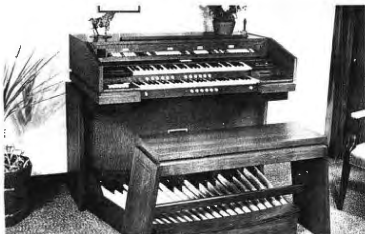
This Allen organ uses digital computer cards to generate different sets of voices.
