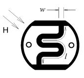
$R_H$  = resistance of cell at light level H
