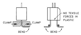
Examples of Tooling Fixtures Used to Form Leads
