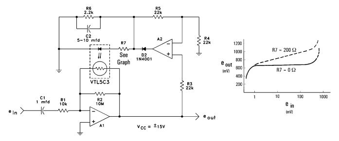
Figure 4a. Peak Sensing Compressor
