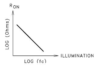
Defining the sensitivity required for a specific application can prove to be one of the more difficult aspects in specifying a photoconductor. In order to specify the sensitivity one must, to some degree, characterize the light source in terms of its intensity and its spectral content.
