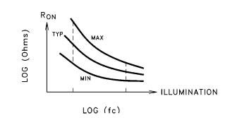
Likewise, for dual element photocells the matching factor, which is defined as the ratio of the resistance of between elements, will increase with decreasing light level.
