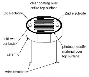
Figure 3 Typical Construction of a Plastic Coated Photocell
