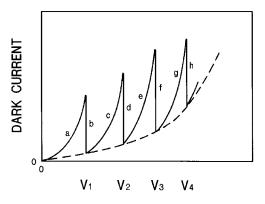
Figure 4. Breakdown characteristics of photocells with low resistivity photoconductive material.
