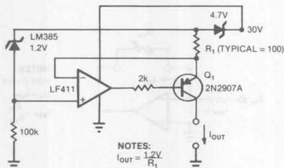
**Fig 3**—Another way to achieve grounded-load isolation is to force the potential across  $R_1$  to equal the LM385's 1.2V reference voltage. This circuit achieves higher voltage compliance than Fig 2's.
