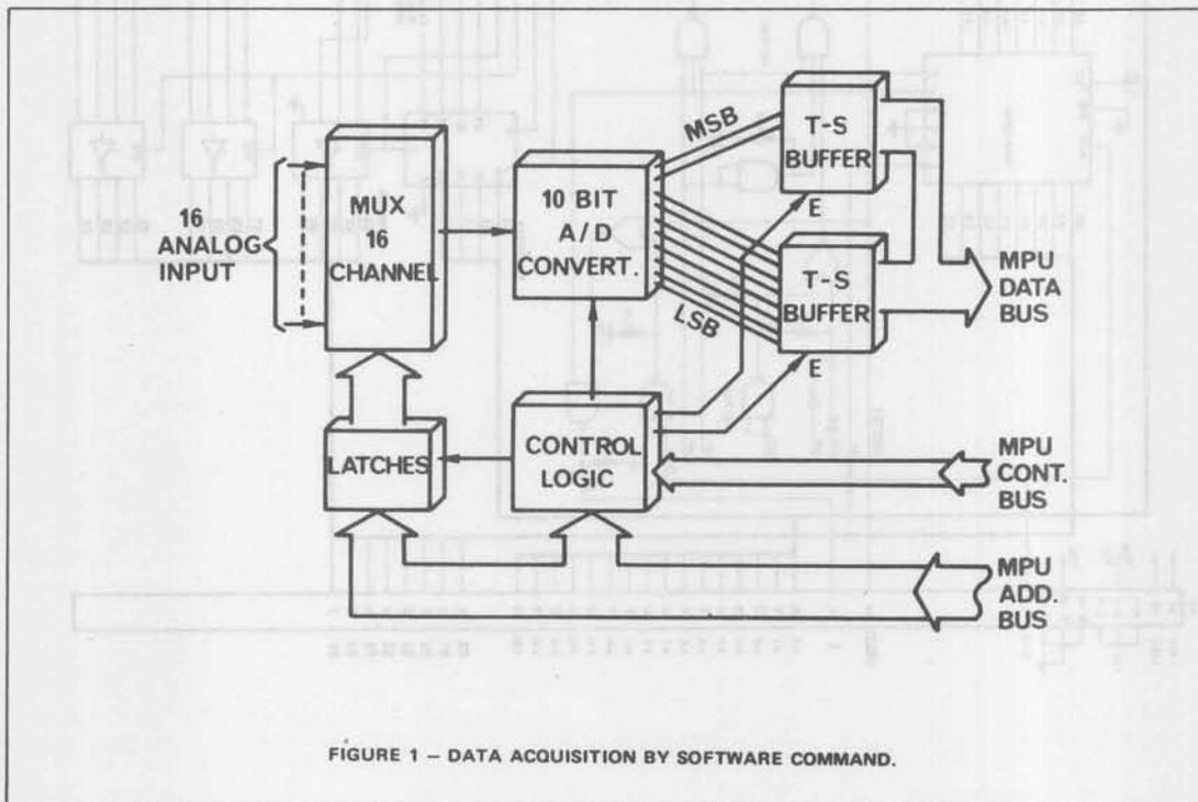
FIGURE 1 - DATA ACQUISITION BY SOFTWARE COMMAND.
