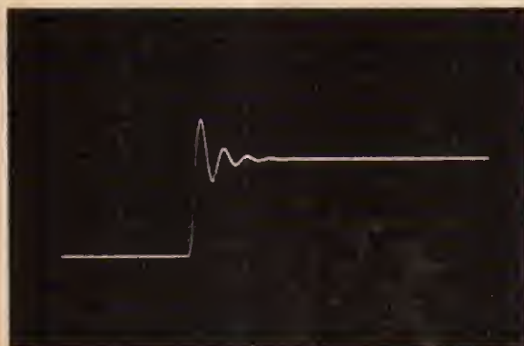
Photo B. Ringing caused by non-selective feedback
