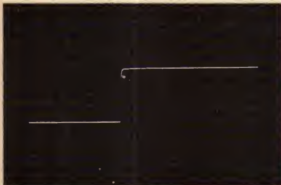
Photo A. Leading edge of the 1kHz square wave
