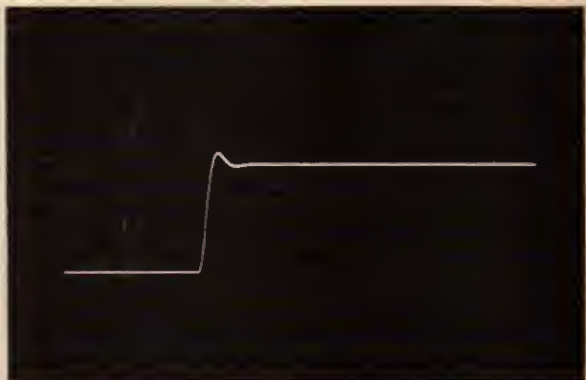
Photo C. Ringing is brought down to an acceptable level by selection of a parallel capacitor across the feedback resistor
