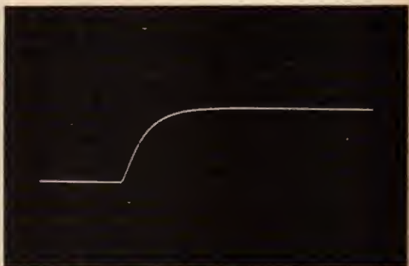
Photo D. Larger value of capacitance increases the rise time
