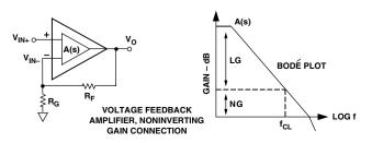
that no current flows into the op amp (infinite input impedance); both inputs will be at about the same potential (negative feedback and high open-loop gain)).
