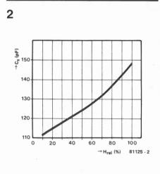
Figure 2. The relationship between relative humidity  $H_{rel}$  and sensor capacitance  $C_s$ .
