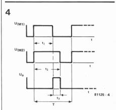
Figure 4. How pulses are formed in the circuit of figure 3. The pulse width determines the degree of humidity H<sub>rel</sub>.
