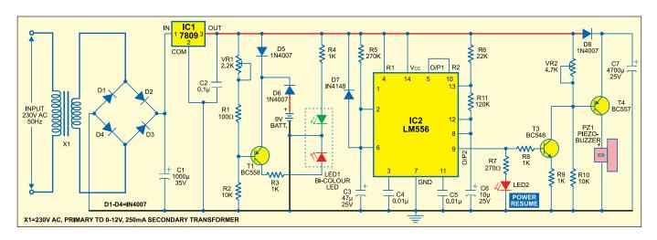
full-wave bridge rectifier comprising diodes D1 through D4, filtered by capacitor C1 and regulated by IC 7809 (IC1) to give regulated 9V DC to operate the circuit.
