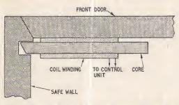
Fig. 3. Sectional plan view of the solenoid bolt mounted inside the safe on the door. Note the chamfered bolt to facilitate easy closure
