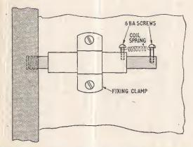
Fig. 4. Interior view of the solenoid balt mounted on the door with a clamp. The coil spring allows the bolt to remain in the "locked" position until operated by the combination circuit
