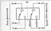
Figure 3. Keyswitch connections
