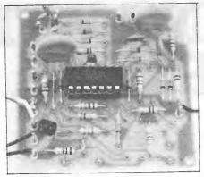
them, fit all sixteen veropins and solder those too. Cut all excess leads and check for dry joints and short circuits. Insert IC1 into the holder and proceed with testing the board.
