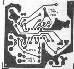
Figure 2. PCB layout and legend
