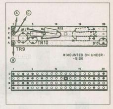
Fig. 7. Veroboard construction of the detector units. Note that point C goes to the jack plug tip.
