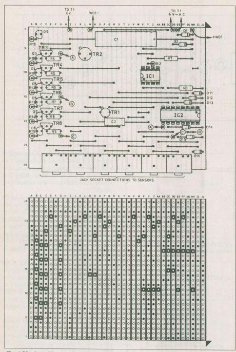
Fig. 4. Veroboard layout and wiring.
