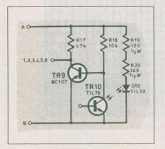
Fig. 3. Circuit of the alarm detector.
