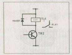
Fig. 2. Addition of a relay to drive other output devices.
