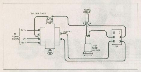
Fig. 5. Supply wiring.
