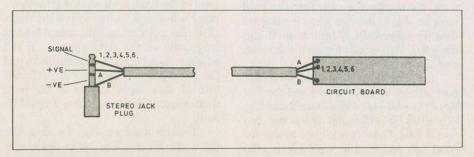
Fig. 9. Wiring of the detectors to the stereo plugs for connection to the master unit.
