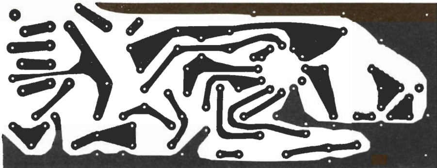
Fig. 2. This actual-size PC board foil layout should be made on a glass-epoxy board, rather than paper-phenolic, to reduce the possibility of poor operation due to stray leakage paths.
