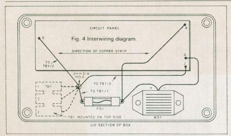
Fig. 4 Interwiring diagram.
