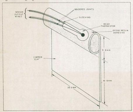
Fig. 5 Mounting and protection of the bead thermistor.
