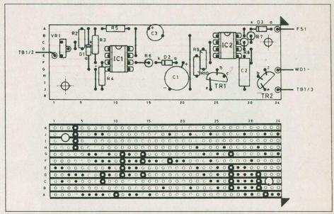
Fig. 3 Veroboard layout and wiring.
