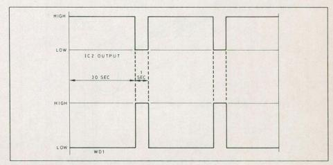
Fig. 2 IC2 output and WD1 drive waveforms.
