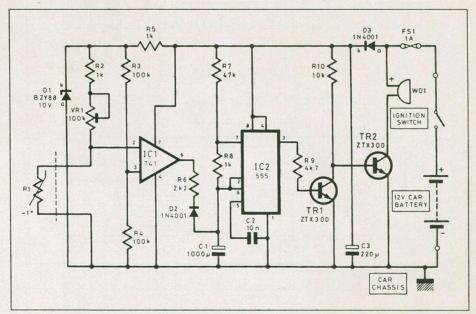
Fig. 1 Circuit diagram of the Thermal Alarm.
