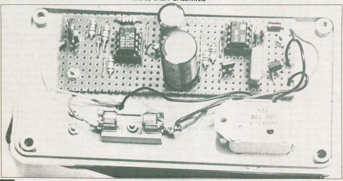
his circuit is designed to detect high temperatures, and has many uses; It could also be useful to readers who experience overheating problems with any car. It is suitable for both positive and negative ground systems.
