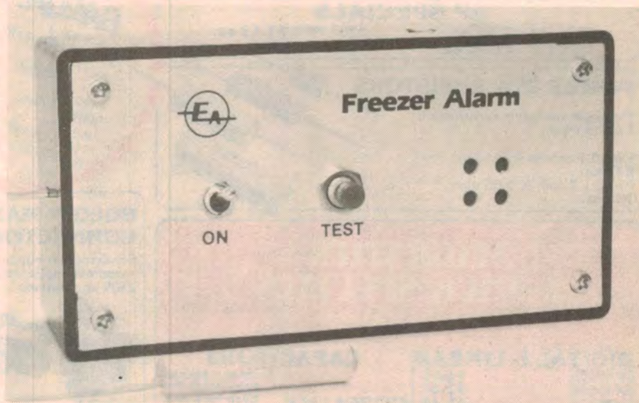
The complete Freezer Alarm is housed in a small plastic box, and the panel we have prepared gives it a professional appearance. The sensing probe, which is normally in the freezer, is shown in front of the box.
