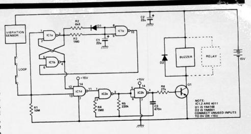
quickly remakes the broken loop or the vibration sensor quickly breaks the loop, the monostable ensures that the alarm continues to sound for approximately 20 seconds. If the loop is left open then the alarm will sound all the time. Unused inputs of the CMOS chips should be tied to V<sub>CC</sub> or 0V whereupon the quiescent battery
