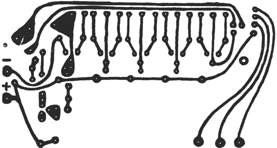
Fig. 2. Foil pattern and component installation for the lock.
