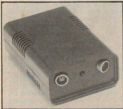
The alternative movement detector version was built into a clip-together plastic case from Dick Smith Electronics.
