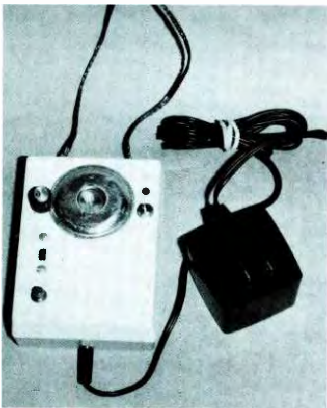
THE PANOPLY and battery charging unit ready to go. The holes required to mount all cabinet-mounted components were cut in the plastic case with a hot soldering-iron tip and awl. Note the coaxial-cable braid at the top of the unit; it is looped around a doorknob to link the knob with the Panoply.
