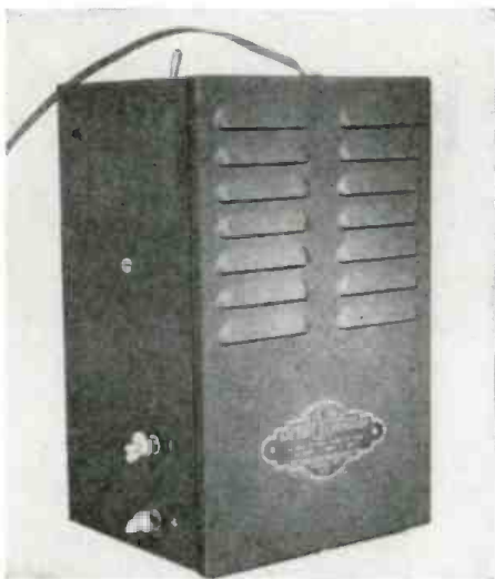
Photo 1—This is original battery eliminator.
