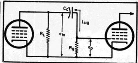
Fig. 8. Equivalent output circuit at low frequencies.  $C_c$  is the deciding factor.
