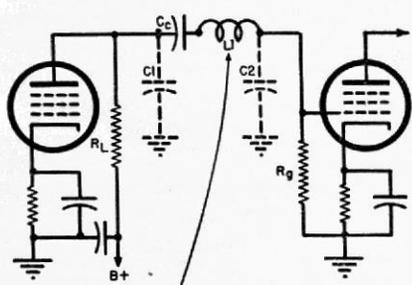
SERIES PEAKING COIL ISOLATES C1 & C2—PERMITS HIGHER RL AND LARGER SIGNAL ACROSS Rg AT HIGH FREQUENCIES
