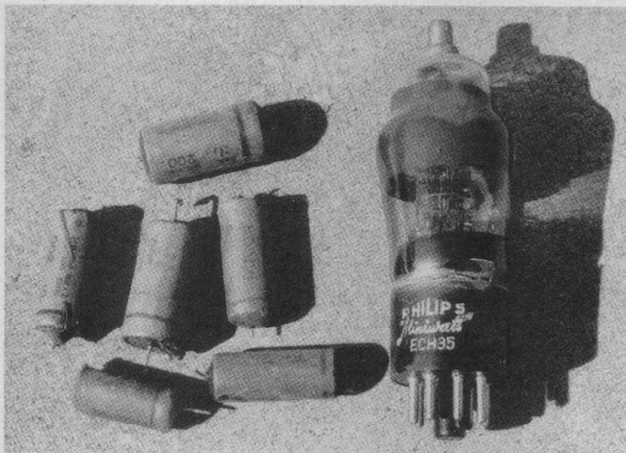
A completely dead ECH35 valve & a few sick capacitors were all that prevented the Philipsette from working.
